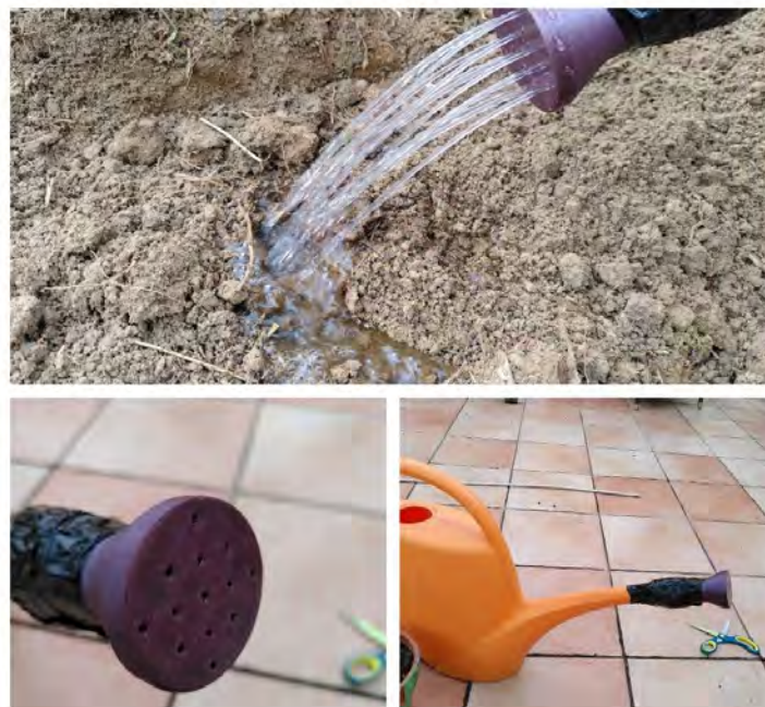
Figure 7: Fixing a watering can with 3D printing.
